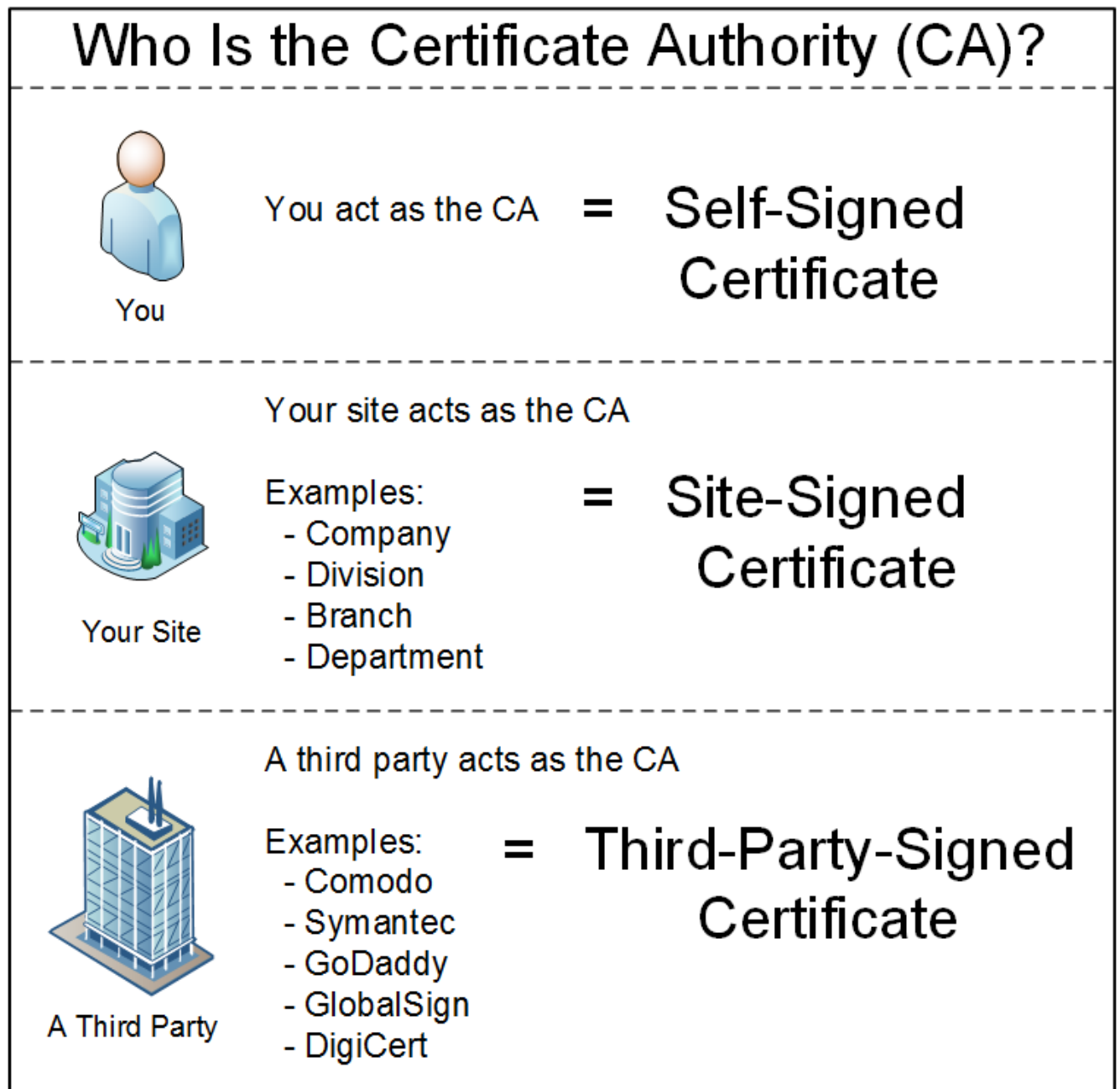
Figure 2 Types of Certificates and Who Acts as the CA for Each Certificate
